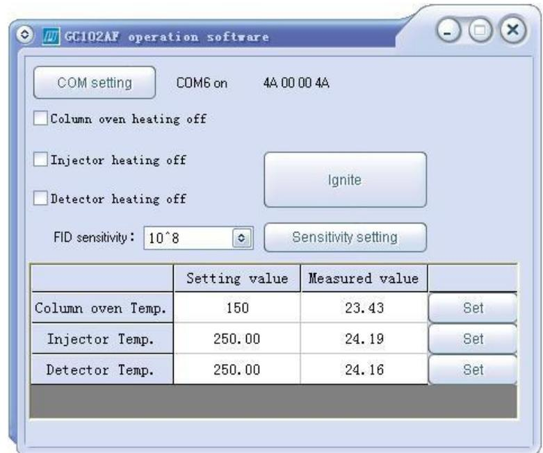
The heating of injector is shut down, the set value of temperature is 250°C and the actual measured temperature is 24.19°C.
