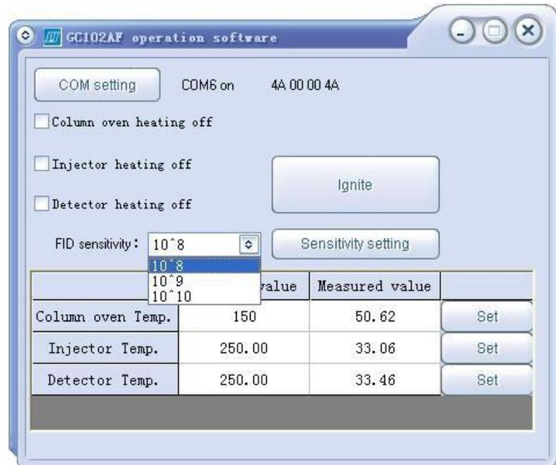
sensitivity:", there are three options:  $10^8$ ,  $10^9$  and  $10^{10}$ . The corresponding FID sensitivity is 10 to 8th, 9th and 10th power, see the right figure:
