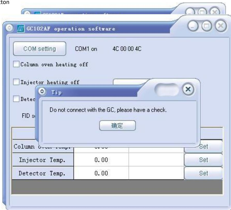
Click the "OK" button to complete the configuration. If the connection is not configured correctly or there is a problem, you can't connect the device. The pop-up window is shown as in the right figure:
